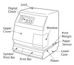
Figure 2-1. Auto-Sync Time Clock External View.
